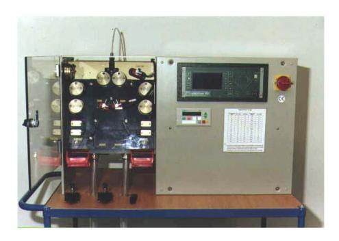
The parts are fed to the test system one after the other in a feeding hose and forwarded unmatched to the test coils by means of two friction wheels.
