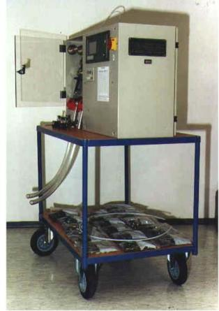
Due to the large wheels of the steel frame the test system can easily be brought to the place of operation. The dust-proof design grants a long operation in production without failure.
