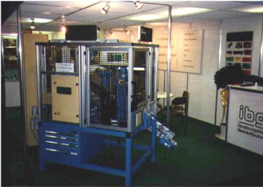
General view with protective grating, tool cabinet and switch cabinet.
