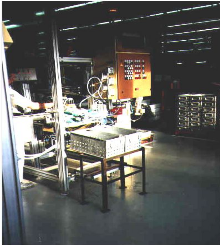
Output NOT O.K. parts: steel box on the right for NOT O.K. (DIMENSION), steel box on the left for NOT O.K. (HARDNESS) and NOT O.K. (CASE DEPTH)
