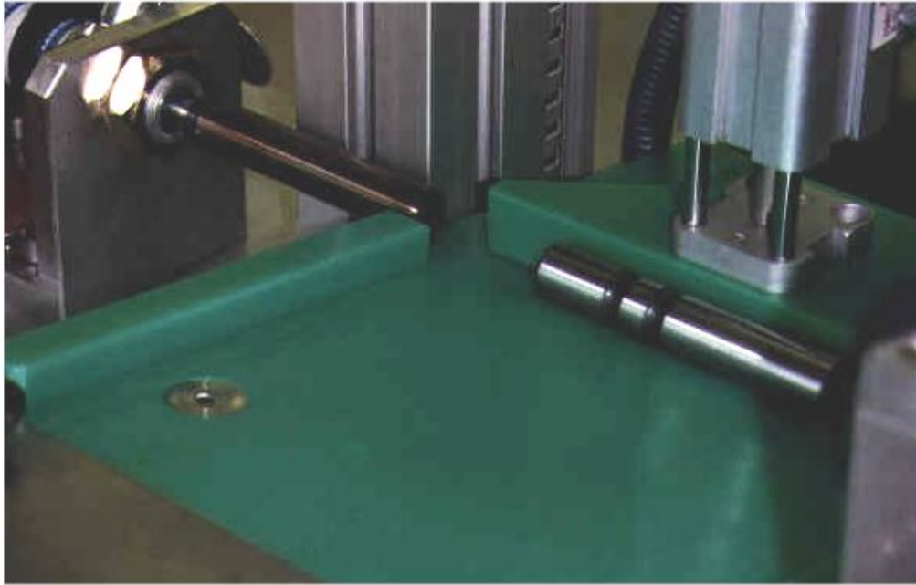
Parts are approaching the stopper for NOT O.K. (DIMENSION) output from the left. Stopper lifts up as soon as sort decision dimension was NOT O.K. The slider (left) pushed the test part into the test coil (to the right).
