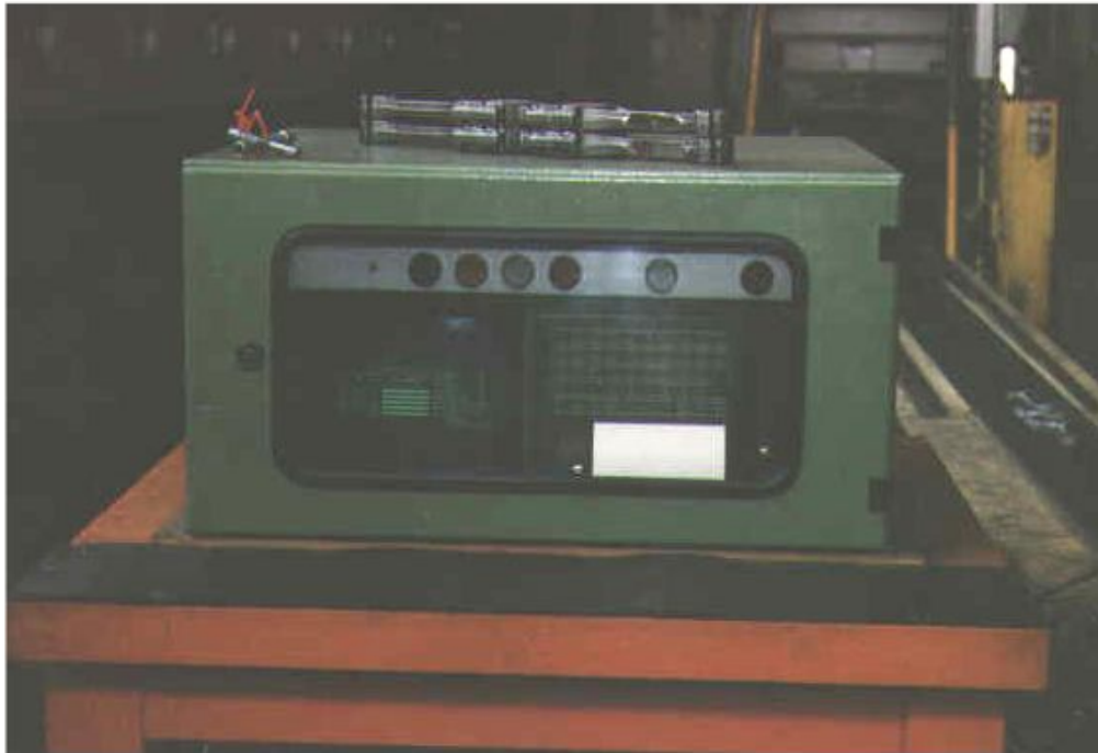
eddyliner ® instrument in robust, dust-proof steel rack
