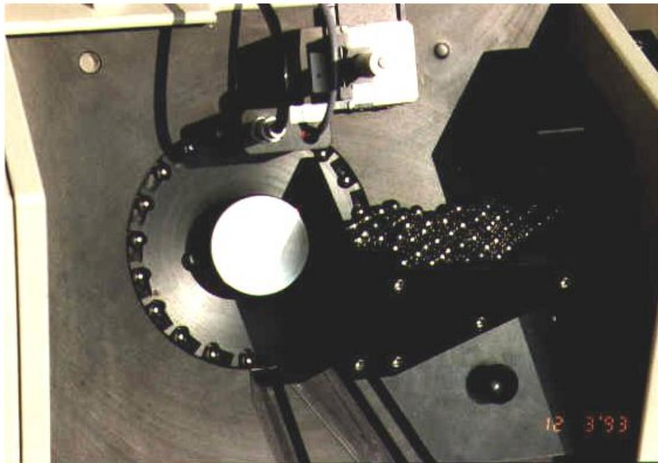
Conveyor disk, bunker, sorting "tongue", sorting channels.
