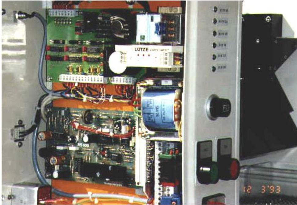
*Speed regulator, shift register, power supply*
