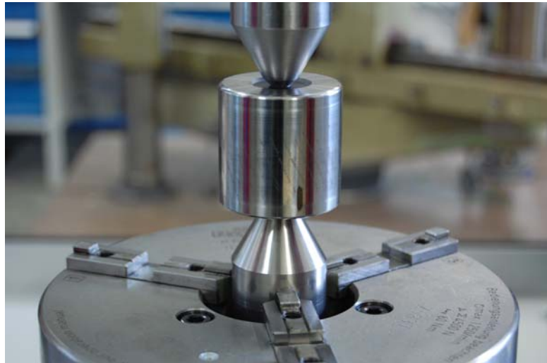
b) Testing a roller
