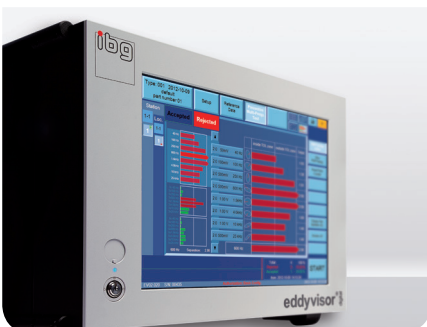
Display of the 3rd harmonic of 1.2 kHz. The measuring results show a good correlation to different induction hardening times.
