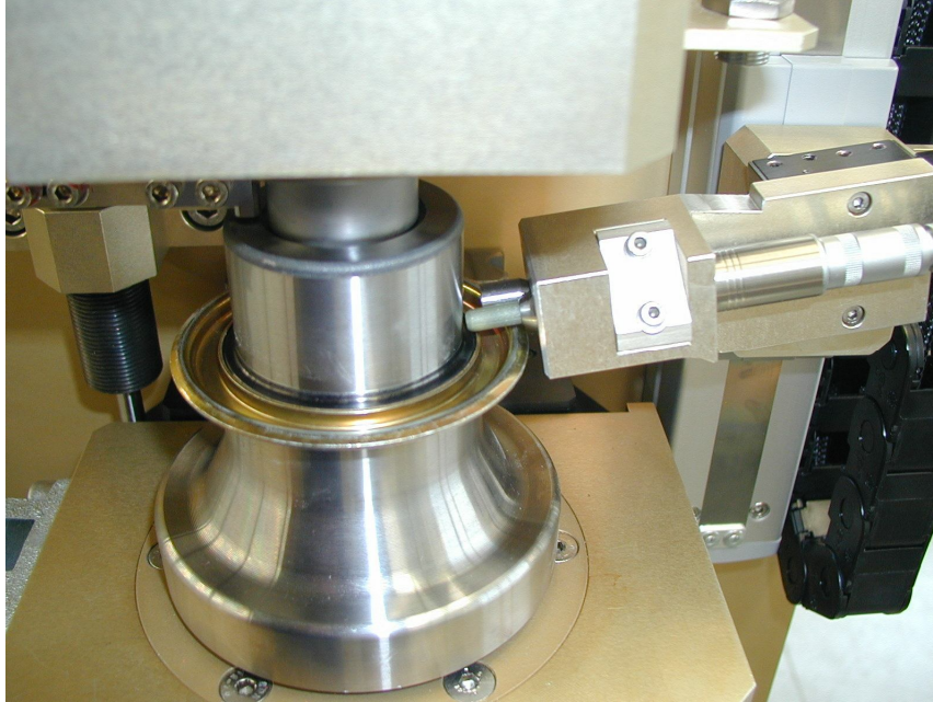
Test position: The test part is scanned for surface-open cracks at the cylindrical outer diameter.
