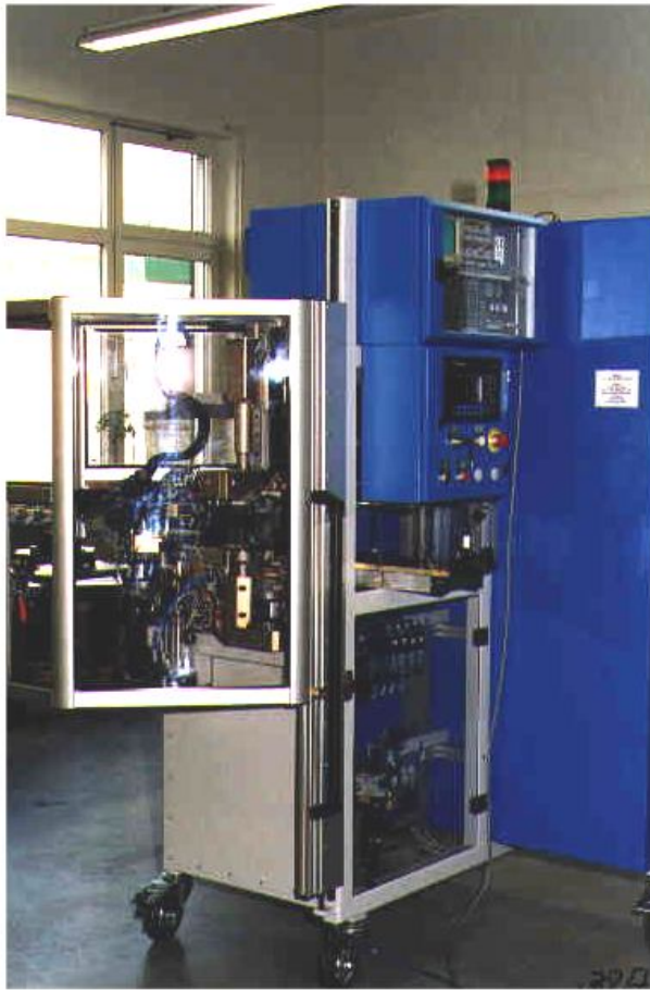
System with closed and opened protective cover (guarantees free access to test station).
