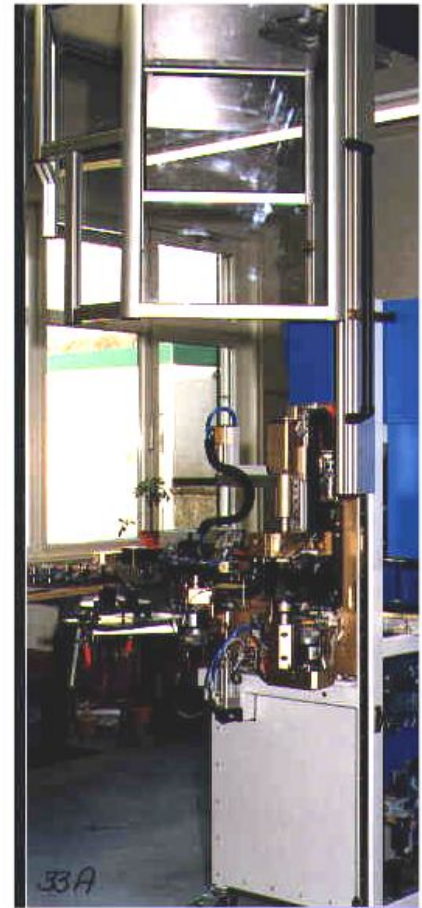
System with closed and opened protective cover (guarantees free access to test station).
