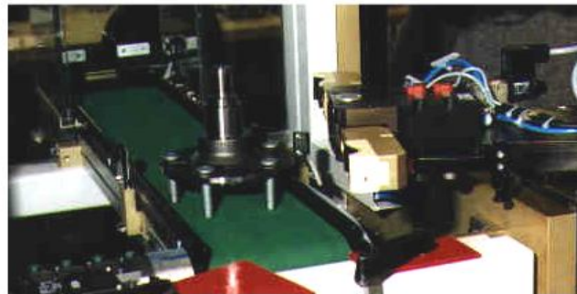
NOK parts are passed on to conveyor belt.
