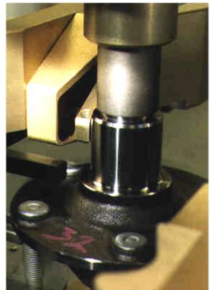
The test probe in the spring-loaded probe-arm scans the whole cylindrical surface, including the radius.
