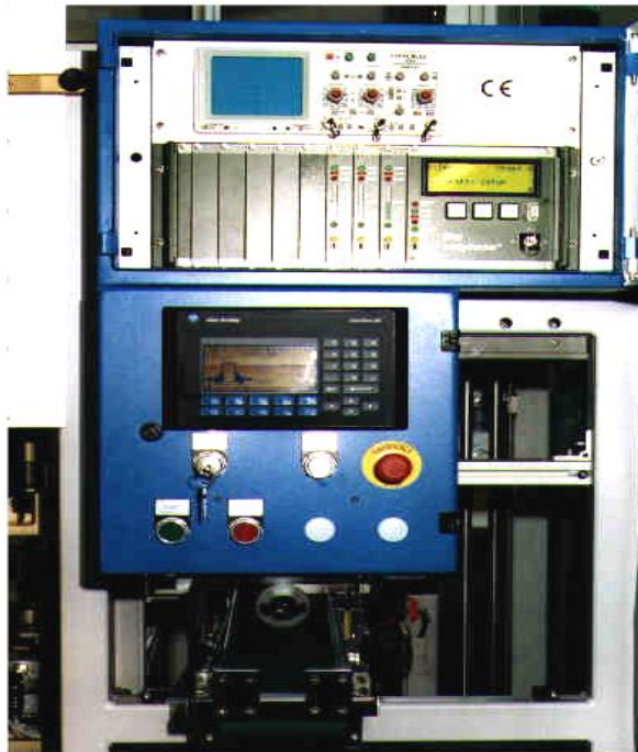
The test instrument, the control panel with graphic user guidance and removal door for NOK parts are easily accesible and well-arranged.
