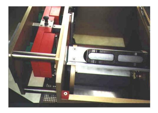
Depending on the sorting decision of the test instrument, the tested part is either forwarded to the OK parts chute via a sorting rocker or passed on to the zincked NOK parts container
