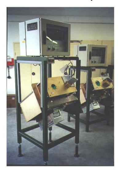
The parts are placed on a parts chute by hand and reach the test position.
