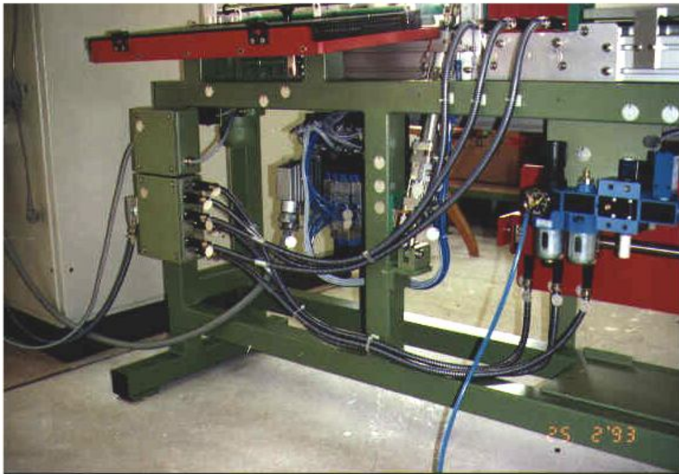
Wiring of pneumatic part, sensor and coils
