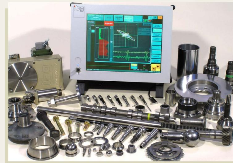
*The basic eddyvisor@SC instrument, in the desktop version, for the testing of material parameters and surface defects.*
