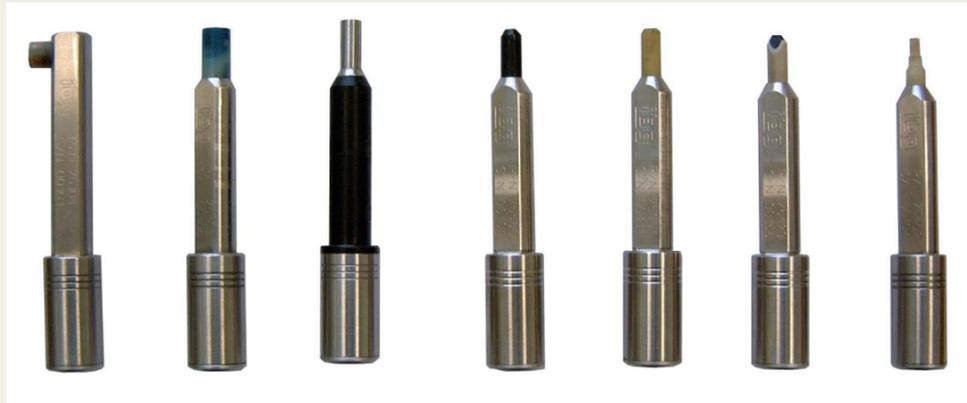
This photo shows a variety of crack test probes.
